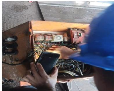
**Gambar 3.13 Memperbaiki *socket relay transfer carriage***
