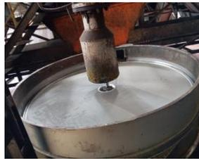
**Gambar 3.80 Penggantian saringan *vibrating screen***
