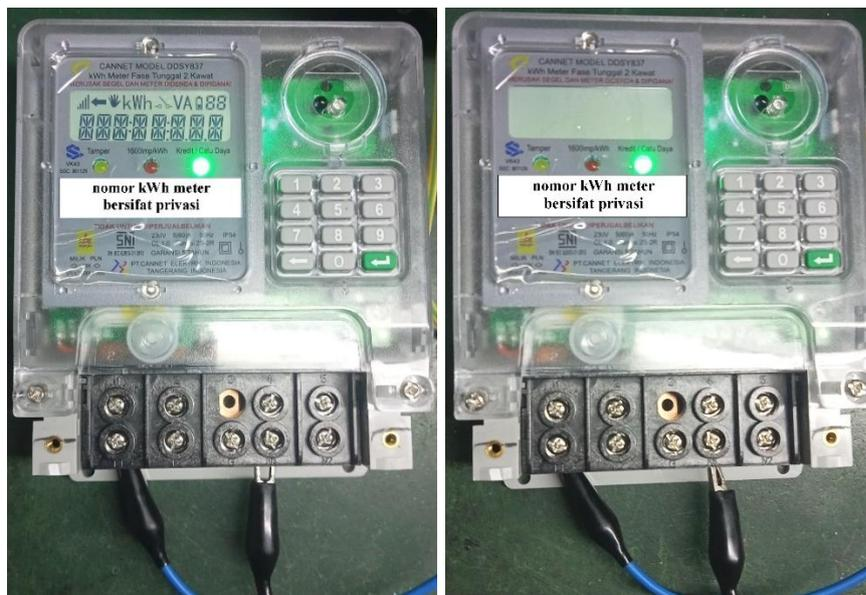
Gambar 3. 7 Contoh Reject LCD Error
