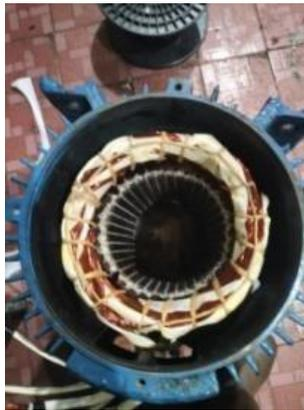
**Gambar 3. 61 Serlak stator elmot transfel line 2**
