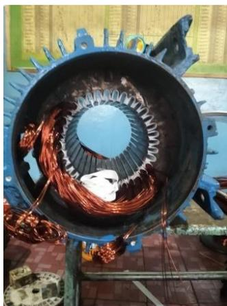
**Gambar 4. 10 Proses renwinding**
