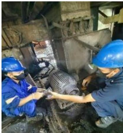
**Gambar 3.14 *Service Elektro Motor Second Dary***
