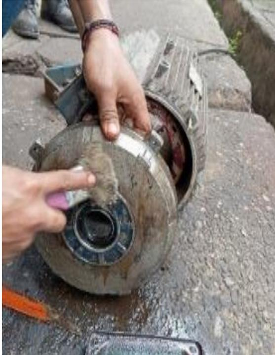
**Gambar 3.37 Membongkar & Pencucian *Sperpart* Elektro Motor Meja *Grading***
