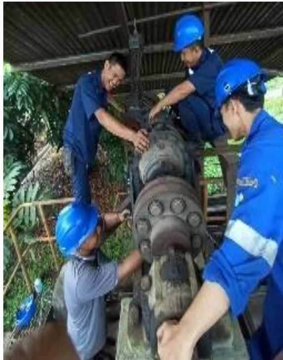
**Gambar 3.86 Perbaikan Seal Elektro Motor Conveyor Loading Ream**
