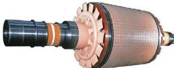
**Gambar 4. 8** Rotor Motor
