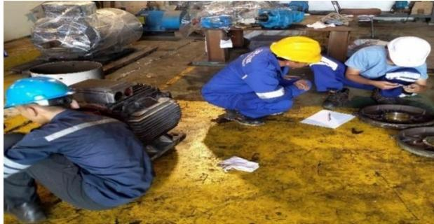
Gambar 3. 40 Pemasangan bearing motor EX C3WP D,E dan N,D,E.
