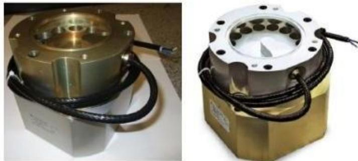
**Gambar 4.1** *Solenoid Operated Gas Admission Valve*
