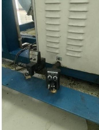
**Gambar 3. 74** *Replace Auto Drain Valve*
