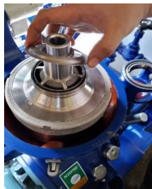
Gambar 4. 8 Gravity Disc (Sumber Dokumentasi: PT. Power Plant)
