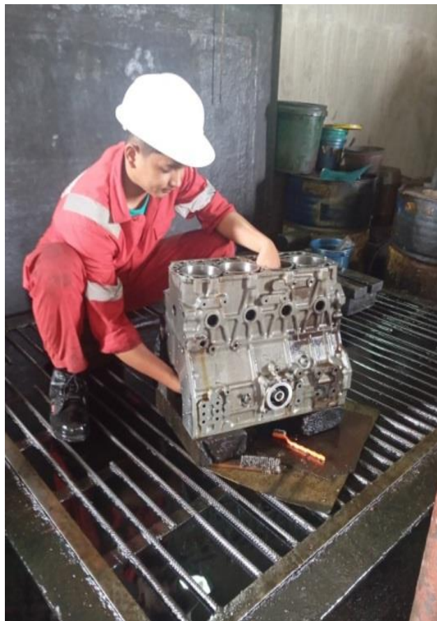
Gambar 3. 3 Pencucian Blok Silinder
