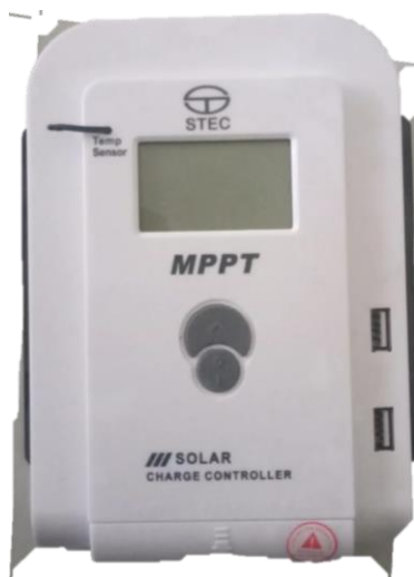
Gambar 3.13 Solar Charger Controller
