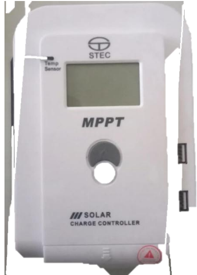
Gambar 3.13 Solar Charger Controller
