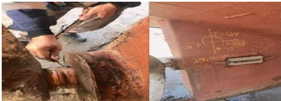
Gambar 2 11 Pengecekan Bantalan As Propeler
