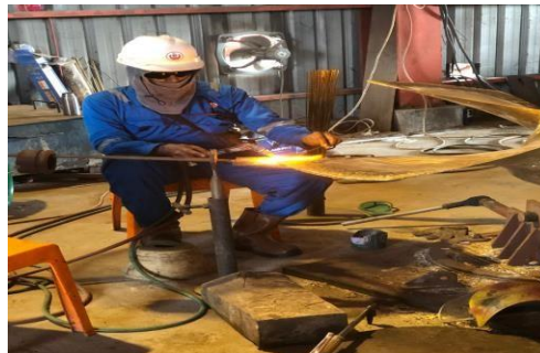
Gambar 3 14 Proses Pengelasan Propeller
