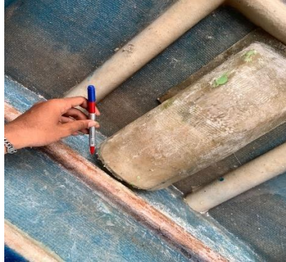
Gambar 4.19 Proses Marking Lubang Nozle dan Intake
