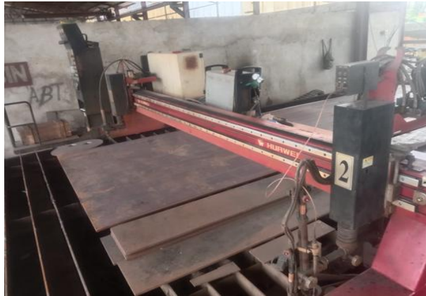
Gambar 3.37 Mesin CNC (Computer Numerical Control)
