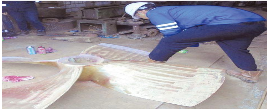
Gambar 2.10 Dye Penetrant Test
