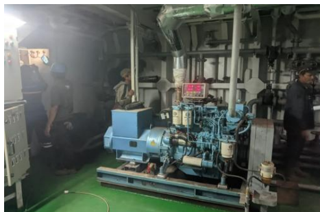
Gambar 3.7 generator diesel dan Main Switchboard
