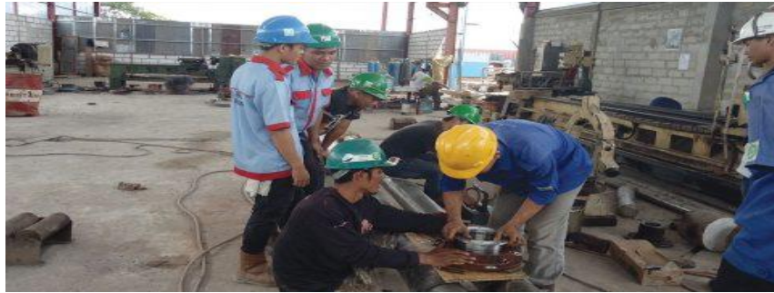
Gambar 2.8 Pengetesan Seal Oil as Propeller Sumber : PT Dutabahari Menara Line Dock Yard
