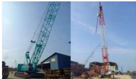
Gambar 2.9 Crawler crane kapasitas 260 ton
