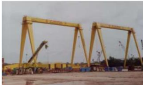
Gambar 2.10 Overhead Crane kapasitas 25 ton
