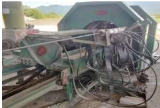
gambar 3.38 mesin cage Forming
