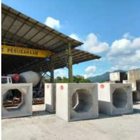
gambar 3.35 box culvert dan u-ditch arean stock
