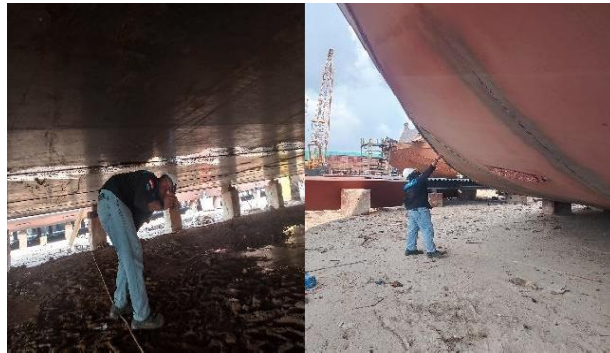
Gambar 3.19 air test & inspect welding
