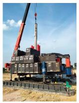
Gambar 3. 2 Hydraulic static pile driver (HSPD)
