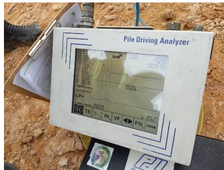
Gambar 3. 43 Alat uji PDA test spun pile
