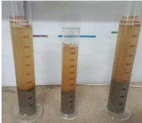
Gambar 3. 5 Pengendapan kadar lumpur agregat halus
