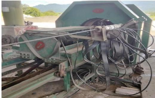
Gambar 3. 36 mesin cage Forming
