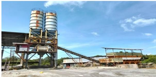
Gambar 3. 35 *Batching Plant*
