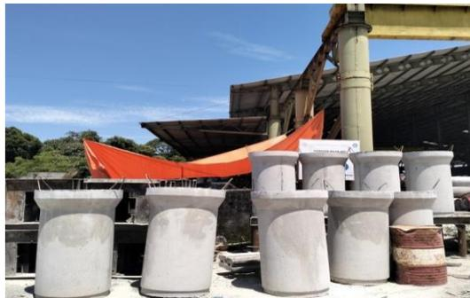
Gambar 3. 32 RCP (*Reinforced Concrete Pipe*)
