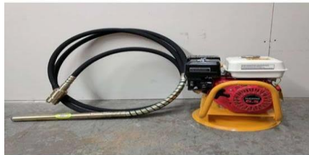
GAMBAR 3. 10 Vibrator concrete machine (Sumber) : Dokumen Lapangan, 2024
