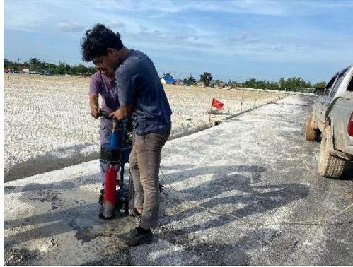
Gambar 3.90 Core Drill Aspal
