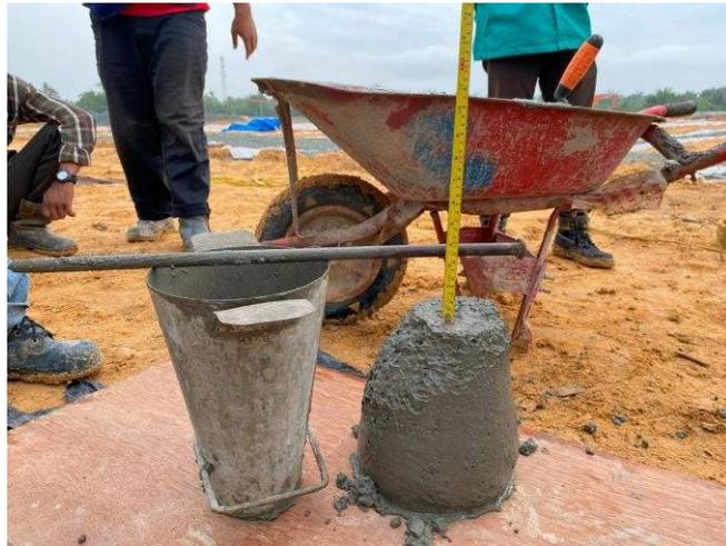
Gambar 3.54 Slump Test
