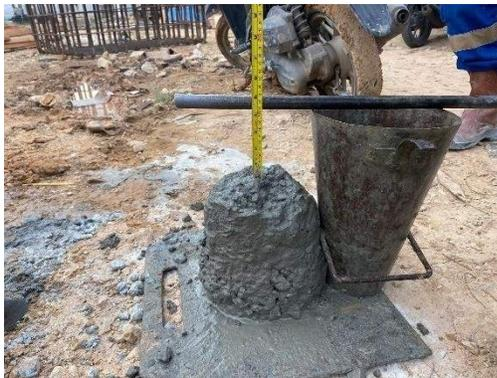
Gambar 3.32 Slump Test
