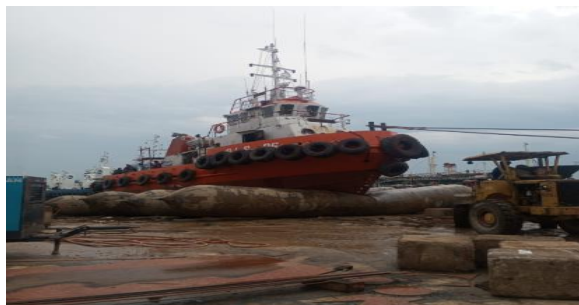
Gambar 3. 58 Proses Launching kapal Pis 05
