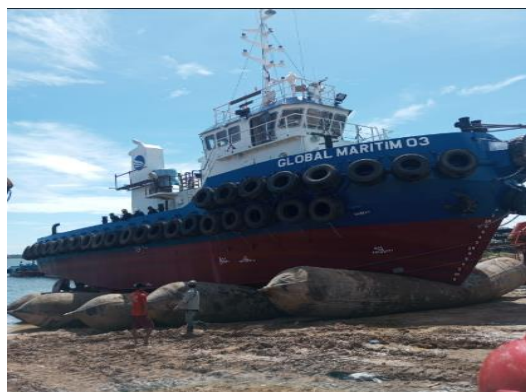
Gambar 3. 39 Launching metode Airbag
