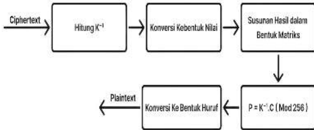
Gambar 2.4 Ilustrasi Proses Dekripsi Hill Cipher [17]
