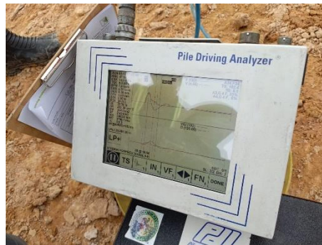
Gambar 3. 43. Alat uji PDA test spun pile
