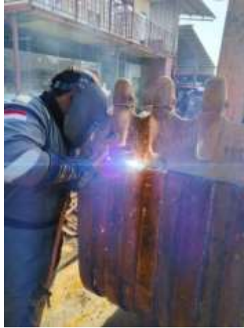
Gambar 3. 18 Mengisi Lasan Bucket Excavator
