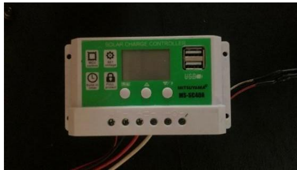
Gambar 2.3 Solar Charge Control Sumber: (Dokumentasi,2026)
