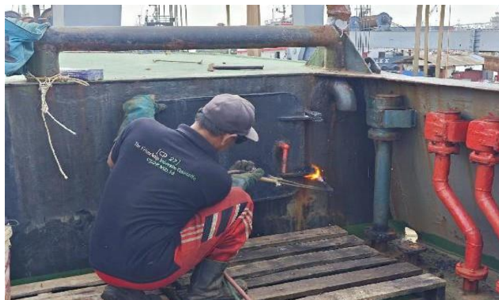
Gambar 4.16 Proses Potong Engsel Hatch Cover Steering Room
