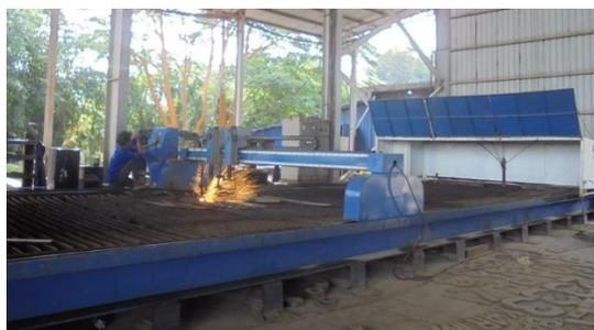
Gambar 1.5 Mesin *Computer Numerical Control (CNC)*
