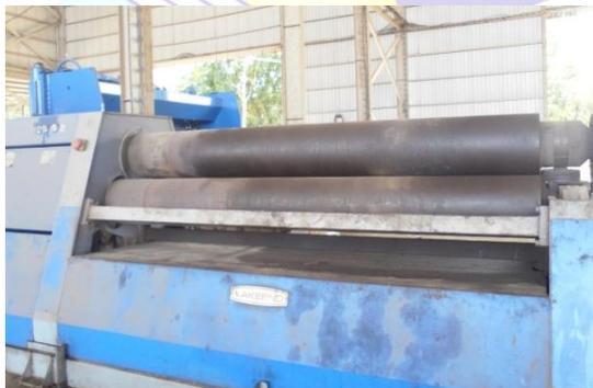
Gambar 1.4 Mesin bending *Roll*
