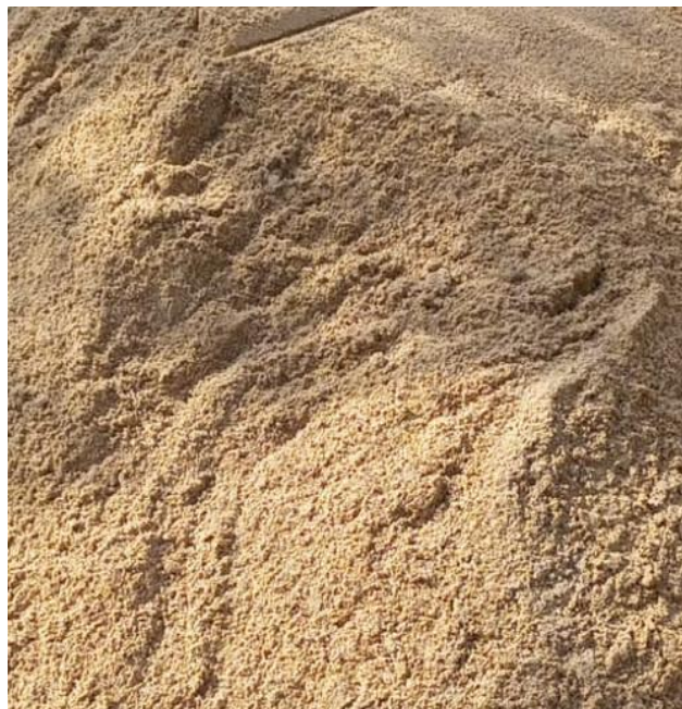
Gambar 4.6 (Agregat Halus) Sumber : Google
