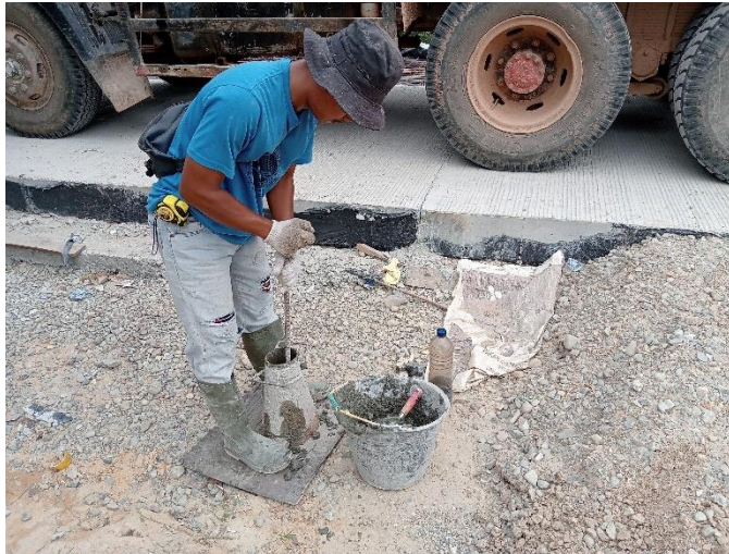
Gambar 4.2 (Proses Penusukan Saat Pengujian Slump)
