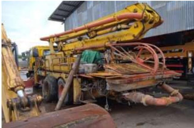
**Gambar 2. 6** Truck concrete pump
