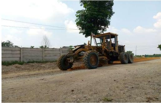
**Gambar 4.3** Motor Grader
