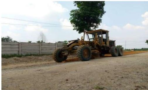
**Gambar 3.4** Motor Grader
