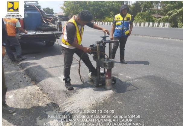
**Gambar 4. 1 Core drill Test**
