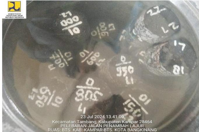
**Gambar 4. 20 Perendaman sampel core didalam ember 24 jam**
