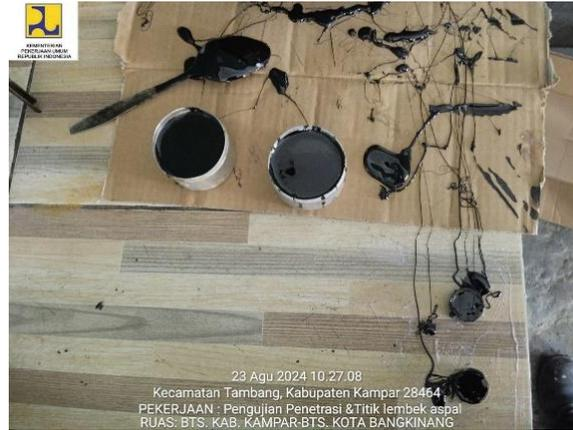
**Gambar 4. 24 Sampel aspal cair didalam wadah**
