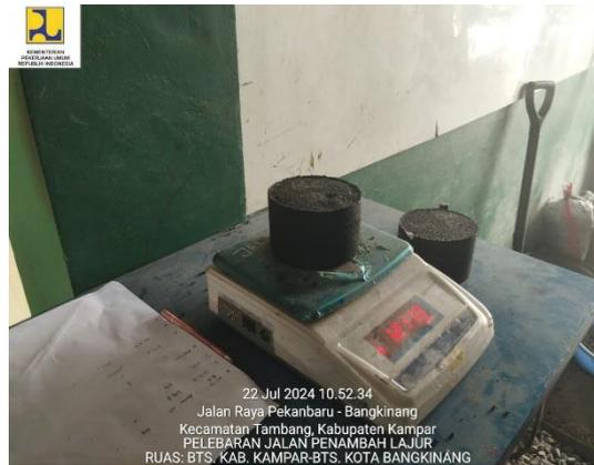
**Gambar 4. 14 Timbang sampel marshal**
