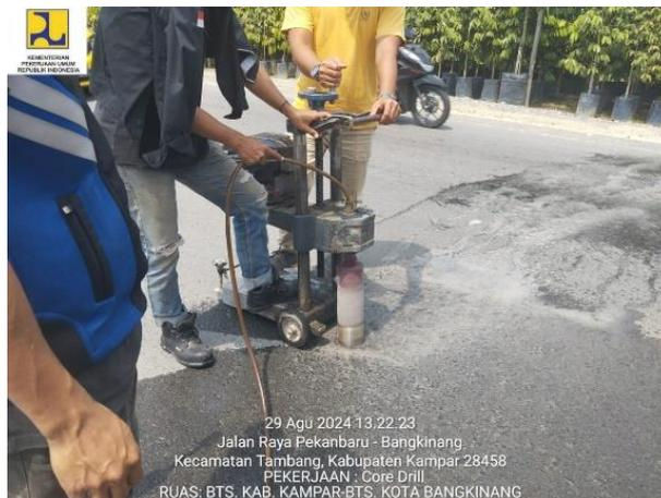
**Gambar 4. 2 Core Drill Test**
