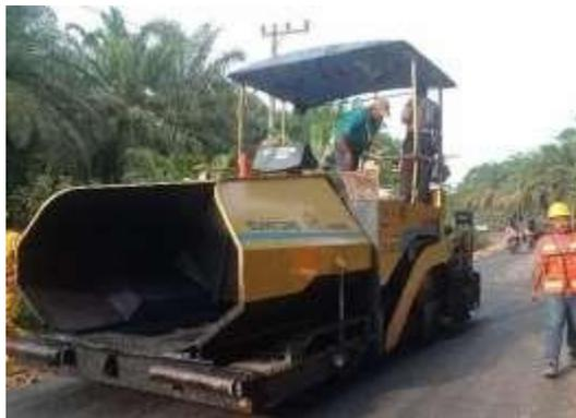
Gambar 3. 4 Asphalt Finisher
