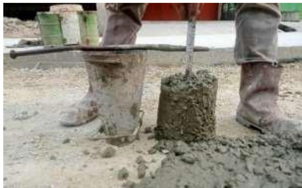
Gambar 3. 31 Pegujian Slump
