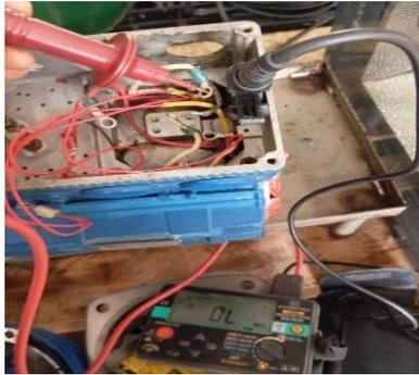
Gambar 4.4 *Resistansi Grounding To Phase*
