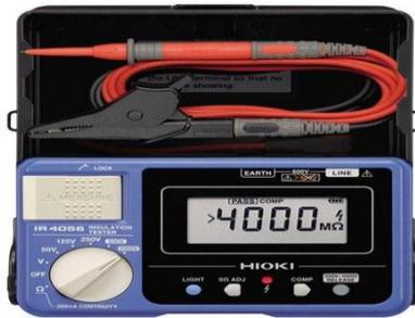
Gambar 3.3 *Megger/Insulation Tester*
