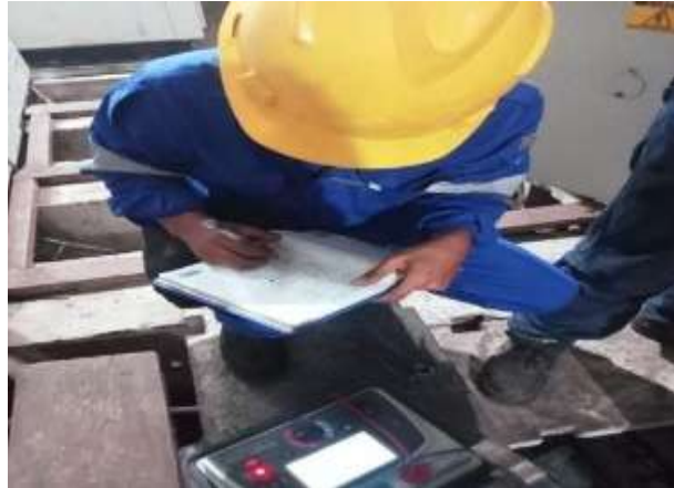
Gambar 3. 65 Magger Motor 6 KV
