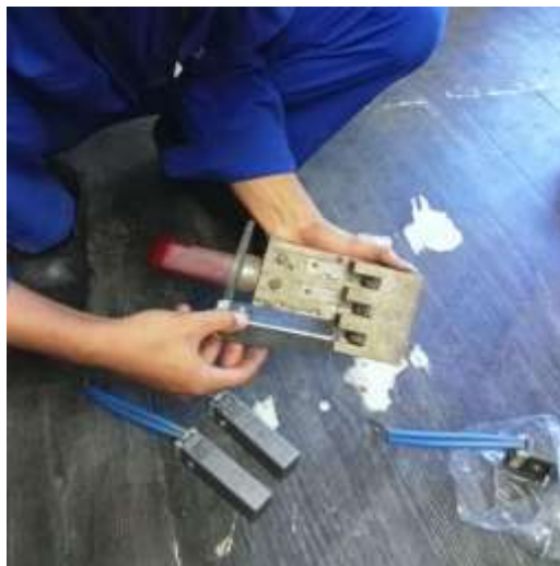
Gambar 4. 21 proses penggantian carbon brush
