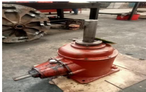
Gambar 4. 10 Gearbox Amarilo F110 Sumber: Dokumentasi,2025
