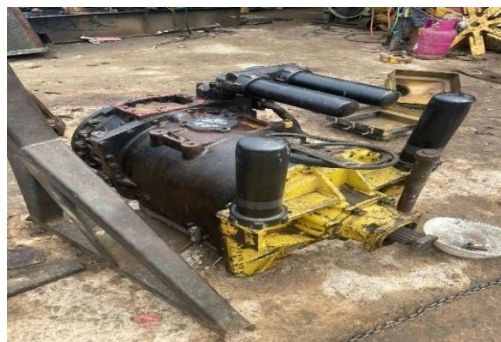
Gambar 3.8 Reassembly transmisi RIG ARJ-05
