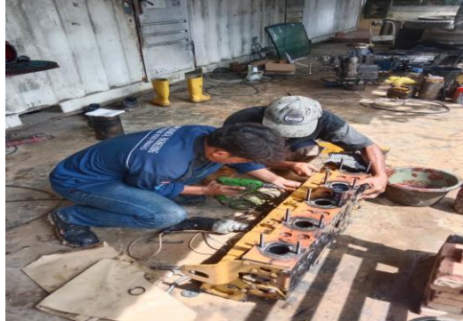
Gambar 3.9 Lapping valve head cylinder Rig-05 (Sumber: Dokumentasi Pribadi)
