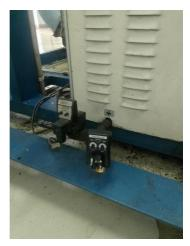
Gambar 3. 74 Replace Auto Drain Valve
