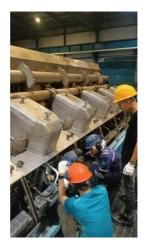
Gambar 3. 64 Pipa Injector
