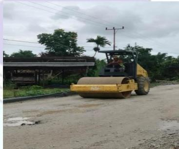
Gambar 3.4: Vibrator roller
