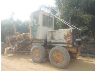
Gambar 3.3: Motor grader
