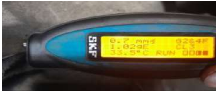
Gambar 4.6 pengecekan vibrasi bearing
