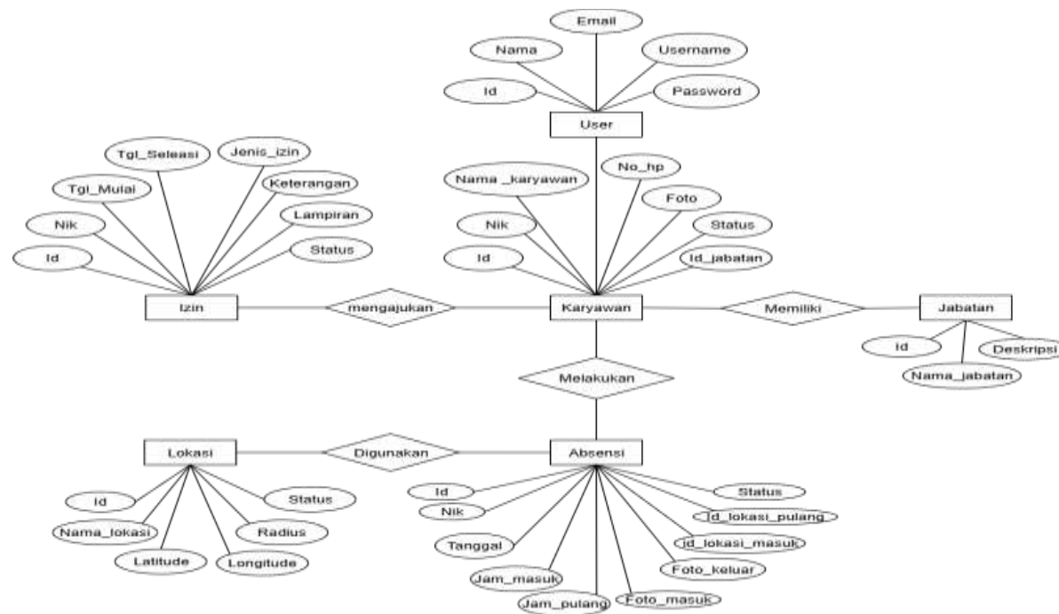
Gambar 4.12 Desain Entity relationship Diagram (ERD)
