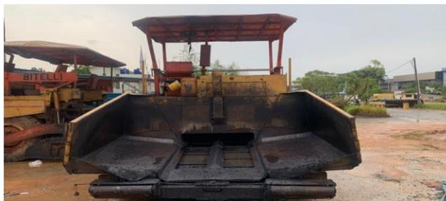
**Gambar 10 - Asphalt Finisher**
