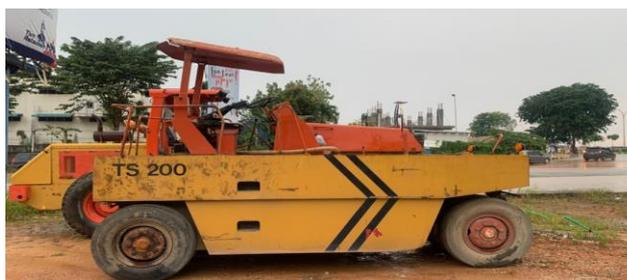
**Gambar 12 - Pneumatic Tier Roller**
