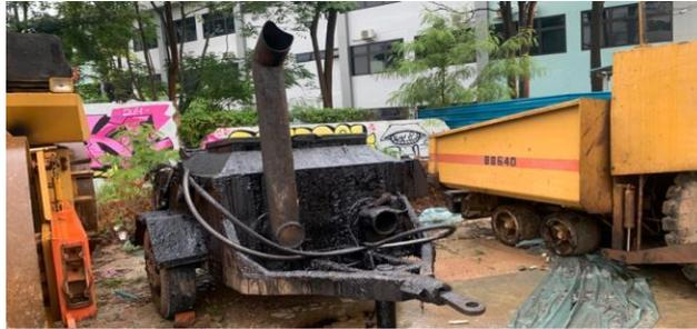
**Gambar 9 - Asphalt Sprayer**
