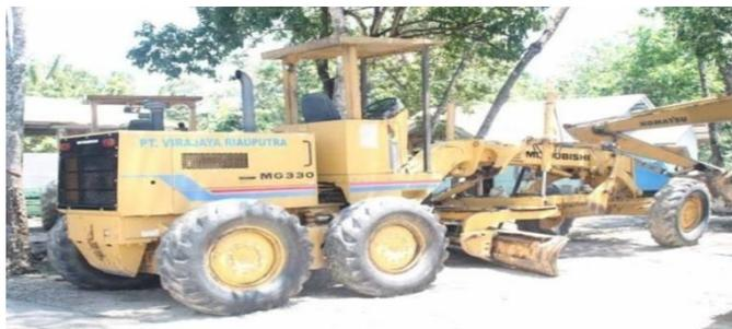
**Gambar 6 - Motor Grader**
