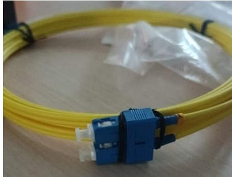
Gambar 4. 22 Kabel patch cord fiber optic tipe SC/UPC duplex singlemode
