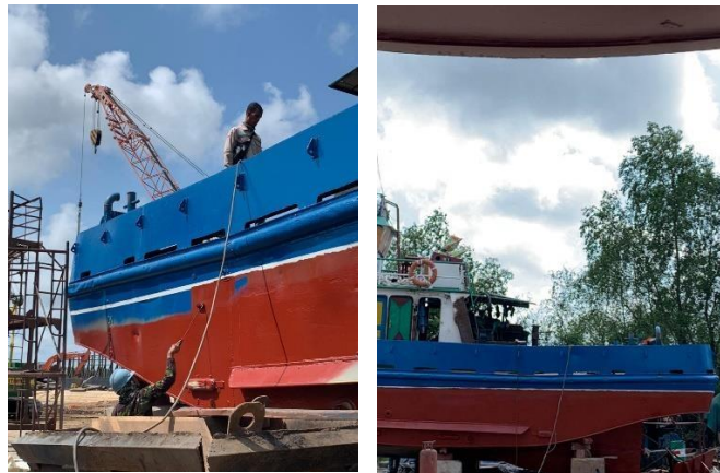
Gambar 3.1. Hasil Pengecatan Anti Korosi Intermediate
