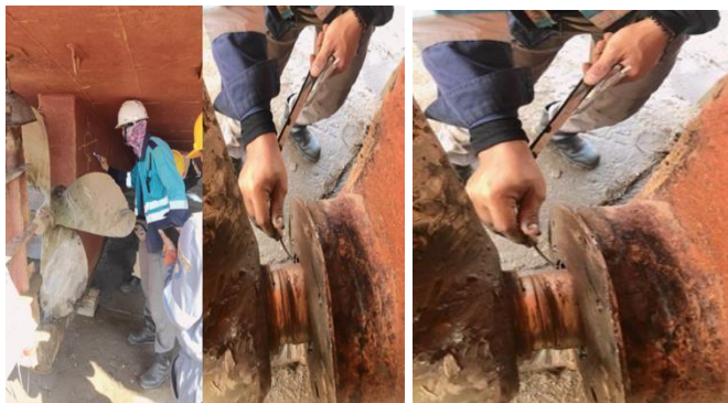
Gambar 2.6 Pengukuran As Propeler
