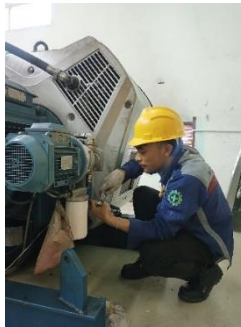
Gambar 3. 19 Filter Compressor Starting
