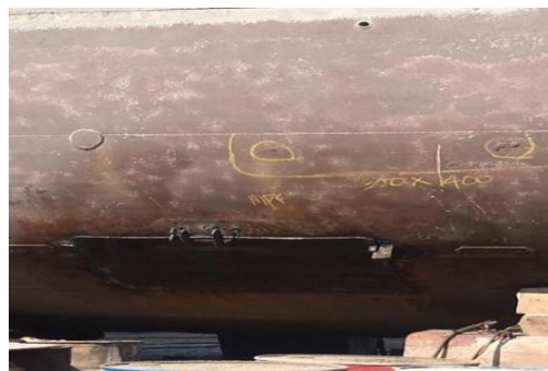
Gambar 2.15 Repleting area bottom&side shell
