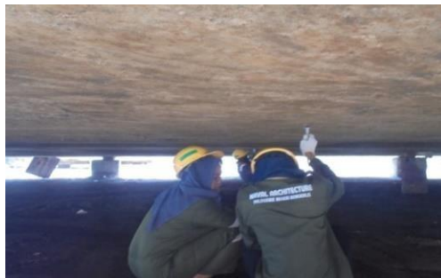
Gambar 2.18 UT thickness area bottom
