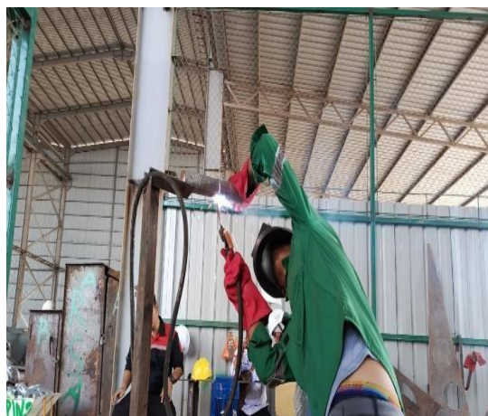
Gambar 2.9 Welder test smaw 5g
