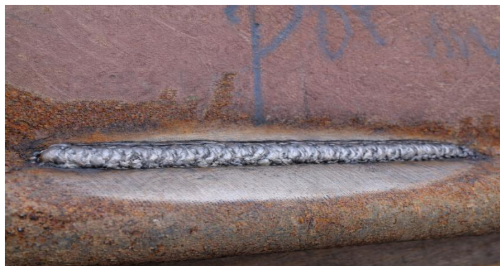
Gambar 4.4 Hasil full re- weld
