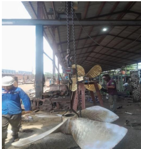
Gambar 3. 26 Penimbangan daun propeler TB.EDWARE 20001
