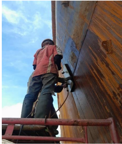
Gambar 3.28 Vakum test TB.JHONI XI
