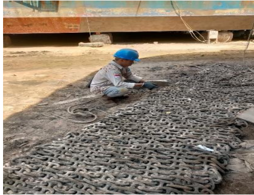
Gambar 3.54 kalibrasi rantai jangkar TB EASTERN STAR
