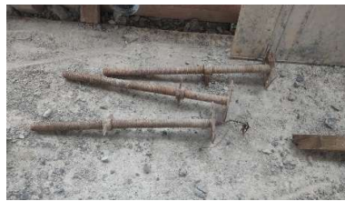
Gambar 3. 26 Base plat scaffolding
