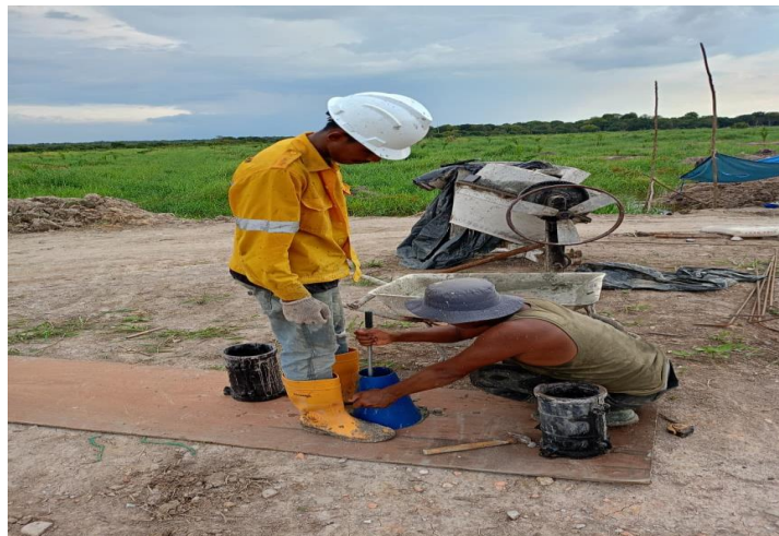
Gambar 3.23 Proses Pengujian Slump Beton
